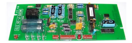
Dinosaur Electronics Replacement Board. Fits the following Dometic refrigerator models: RM2602, RM2603, RM2802, RM2803. The board comes configured to work in 3-way refrigerators and a jumper can be cut to make it work in 2-way refrigerators.
