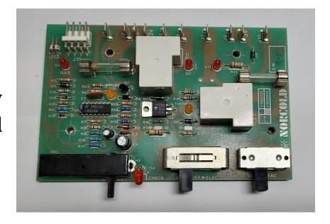
Refrigerator Power Supply Circuit Board; Replacement For Norcold Refrigerator Series 876 EG3\ 878 EG3; 3 Way
